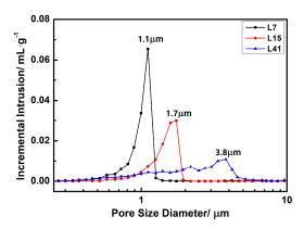
**Figure 2.** Pore size distribution of porous L-SiC ceramics with different particle sizes of the initial coarse SiC powder.
