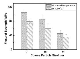
**Figure 4.** Three-point flexural strengths of porous L-SiC ceramics with different particle sizes of the initial coarse SiC powder at normal temperature and 1000 °C.
