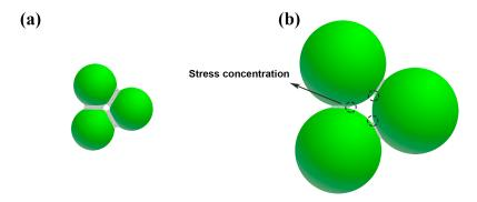
**Figure 5.** Schematic illustration of the sintering neck in porous L-SiC ceramics from (**a**) small particles and (**b**) large particles.
