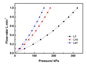
**Figure 6.** Nitrogen gas permeability of porous L-SiC ceramics with different particle sizes of initial coarse SiC powder.
