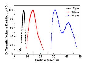
**Figure 1.** Particle size distribution curves of ~7, ~15, and ~41  $\mu m$   $\alpha$ -SiC powders.
