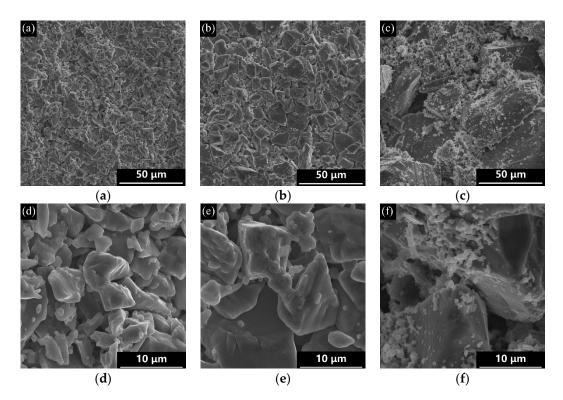
**Figure 3.** SEM images of porous L-SiC ceramics with different particle sizes of initial coarse SiC powder: (**a,d**) 7 μm; (**b,e**) 15 μm; (**c,f**) 41 μm.
