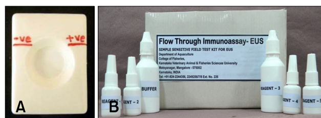
Fig. 2. Images of the flow-through immunoassay (FTA). (A) Nitrocellulose membrane in the cassette. (B) Test reagents.
