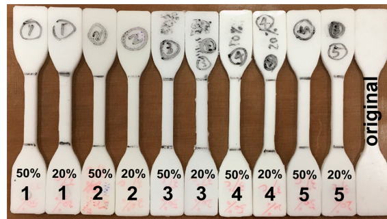
Figure 9. SPPM samples after heated at 50 °C for five minutes. In each sample, the applied programming strain is indicated at right above the hybrid type (1 to 5). The right sample is original as marked without any testing for comparison.
