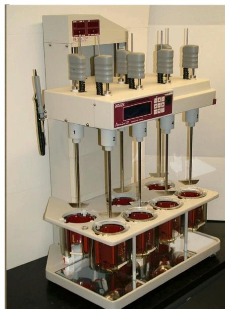
Fig. 2. Distek™ Evolution 6100 Bathless Dissolution System used in this work.
