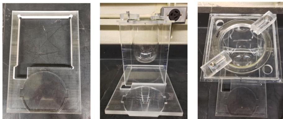
Fig. 3. Custom-made plexiglass square tank base (left panel), and square tank/vessel assembly (center and right panel).
