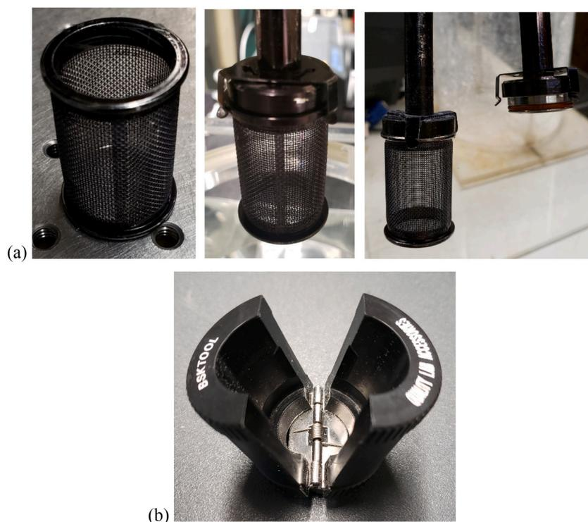
Fig. 5. (a) Dissolution basket (left panel) and details of the three-pronged clip securing the basket to the shaft (center and right panels); (b) Basket grabber (QLA).
