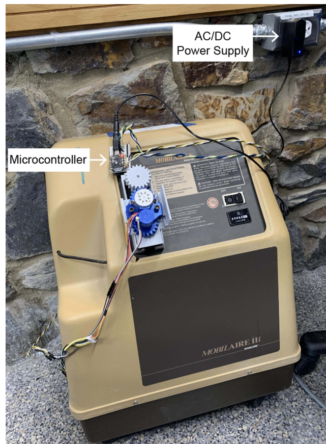
Figure 4 Full concentrator attachment view with electronics plugged into the 110V wall outlet.
