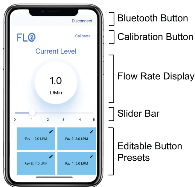
Figure 5 FLO2 application home page with current flow rate display, Bluetooth button, and calibration button. Users can adjust the flow rate by 1) sliding the slider bar to any 0.5 increment value between 0 and 5 LPM or 2) selecting one of the four editable button presets.
