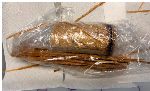
Figure 10. S-3 sprayed bamboo samples covered in a plastic wrap so that the S-3 stays in contact with the impregnated bamboo.
