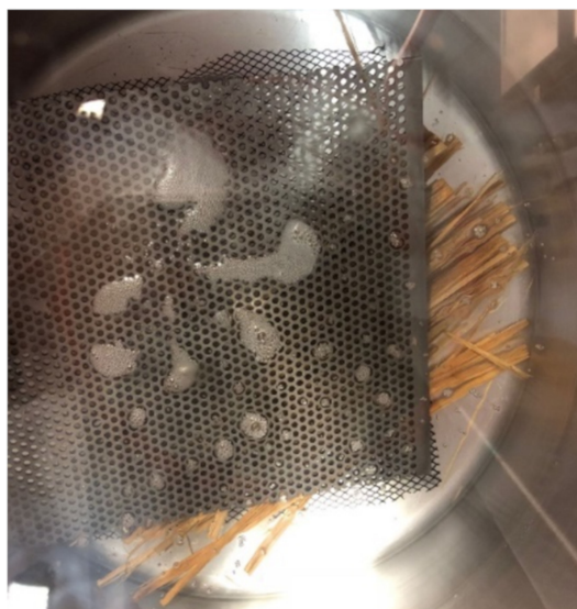
Figure 9. Bubble formation in the silicone chamber due to vacuum pressure reduction.
