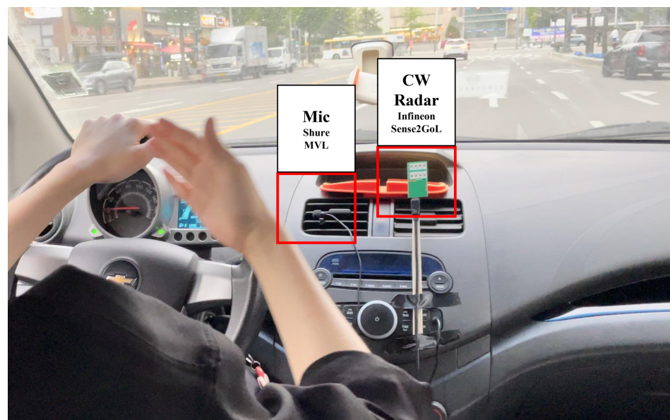
Figure 6. Experiment setup for voice and hand gesture recognition in vehicle.
