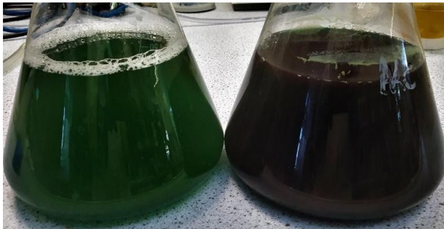
Figure S3: Spirulina biomass solution before (left) and after (right) HC treatment.
