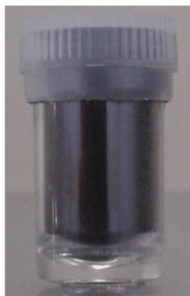
Figure 4. Picture of the natural Molybdenum powder contained into the plexiglass vial used during 14 MeV neutron irradiation at FNG.
