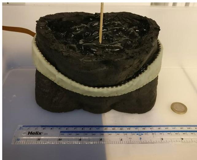
**Figure 2.** Phantom experimental setup. The bladder is submerged in ultrasound gel within the anterior region of the phantom. Further details on the experimental setup are available in Dunne *et al.*<sup>22</sup>.
