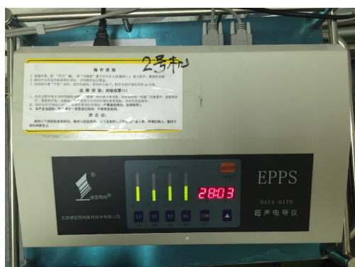
Figure S1 The NAVA-01TD ultrasound and electric pulses for transdermal drug delivery.
