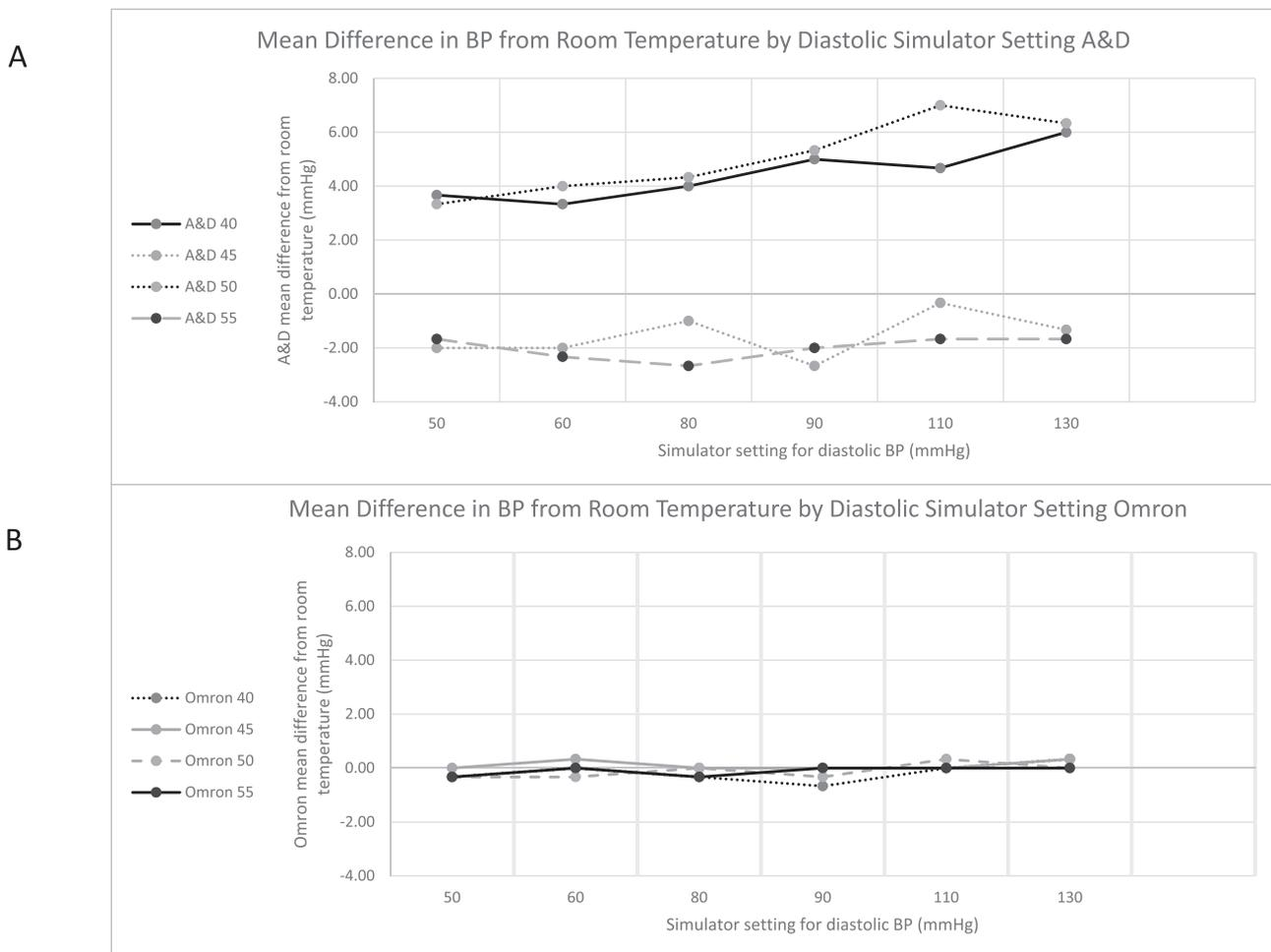
**Figure 2.** Mean differences in BP (elevated temperature minus room temperature), by diastolic BP simulator setting. (a) A&D device. (b) Omron device. Abbreviation: BP, blood pressure.
