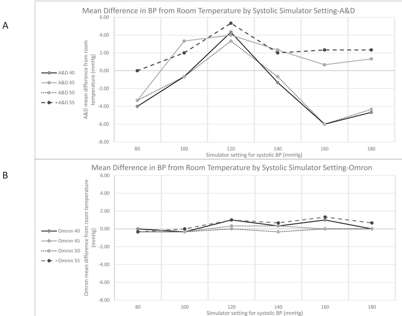
**Figure 1.** Mean differences in BP (elevated temperature minus room temperature), by systolic BP simulator setting. (a) A&D device. (b) Omron device. Abbreviation: BP, blood pressure.
