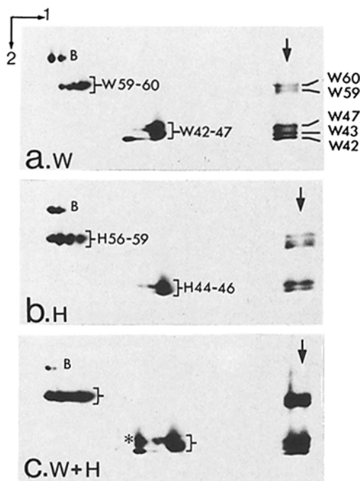
Figure 8. Two-dimensional polyacrylamide gel electrophoresis of keratins from (a) sheep wool, (b) human hair, and (c) a mixture of human hair and wool. Symbols are identical to those of Figs. 4 and 5; asterisk denotes the shift of some acidic keratin toward the basic end, possibly due to complex formation (Franke et al., 1983). Note the striking similarity between human hair and sheep wool keratins.
