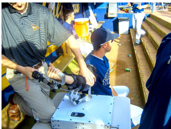
Fig. 3 Testing volunteer with the Elbow Tester
