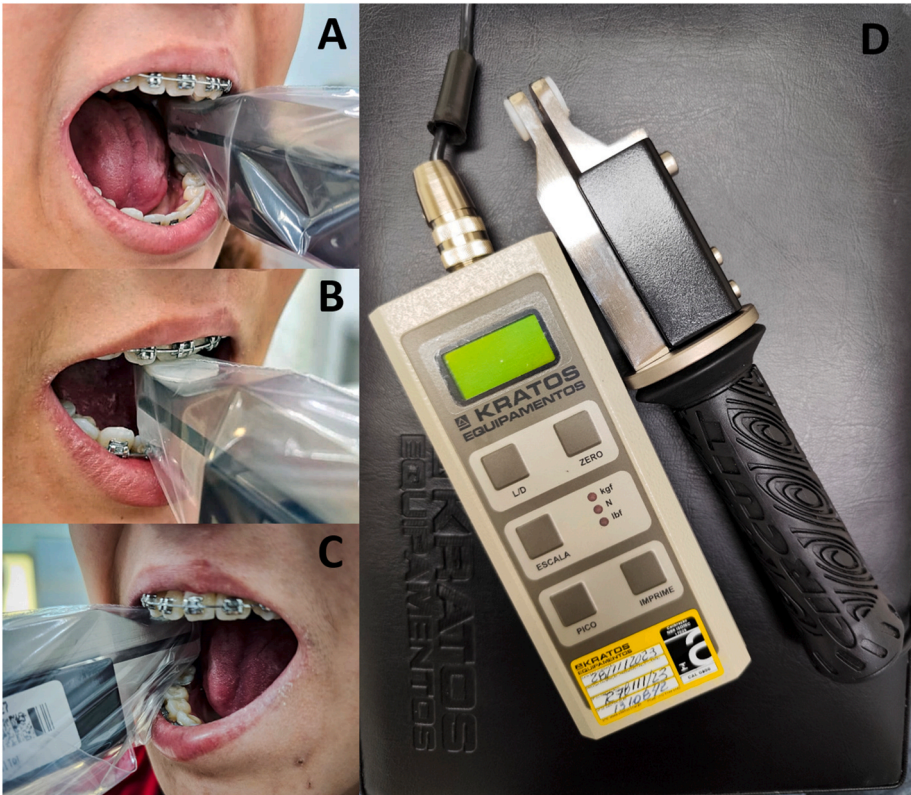
Fig. 2. Positioning of the gnathodynamometer in the regions where bite force was measured. for the CON and CLP group. 2A: left posterior region of the maxilla; 2B: anterior region of the maxilla; 2C: right posterior region of the maxilla; 2D: gnathodynamometer used to perform the measurements (digital dynamometer, IDDK model, Kratos, Bauru, SP, Brazil).
