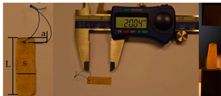
Figure 13. Suture retention strength sample preparation.
