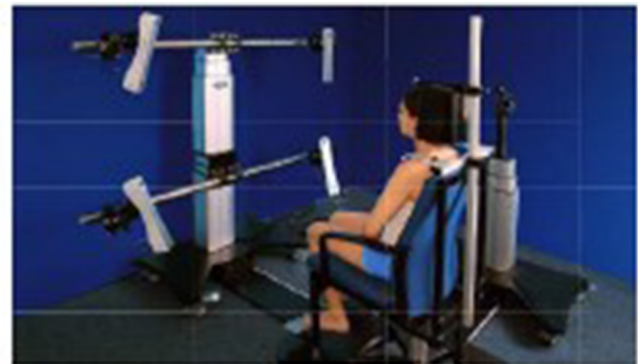
Figure 2 FaceScan system used for facial contour (volume) measurements.
