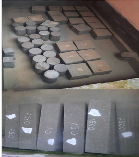
Fig. 4. Wet curing condition of the test specimens.
