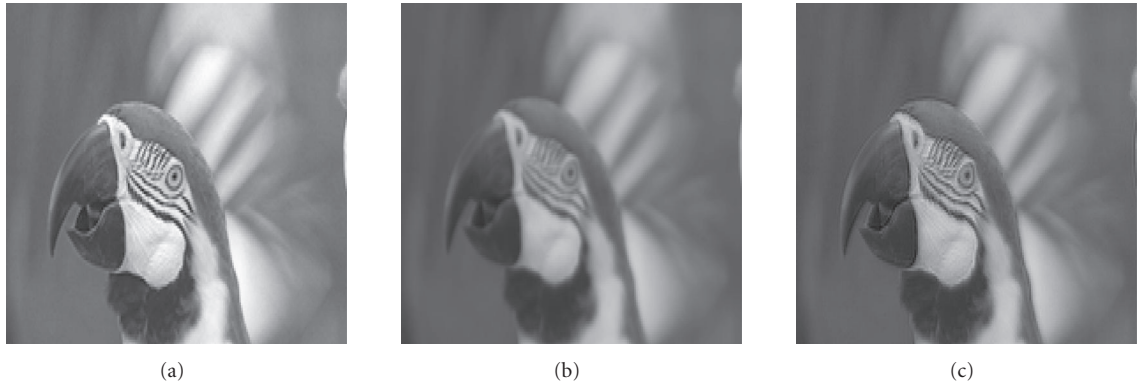
FIGURE 9: Zoomed parrot images for deblurring process: (a) original; (b) blurred; (c) processed.
