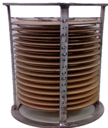
Figure 1. Polymer pressboard specimens used in our experiments.
