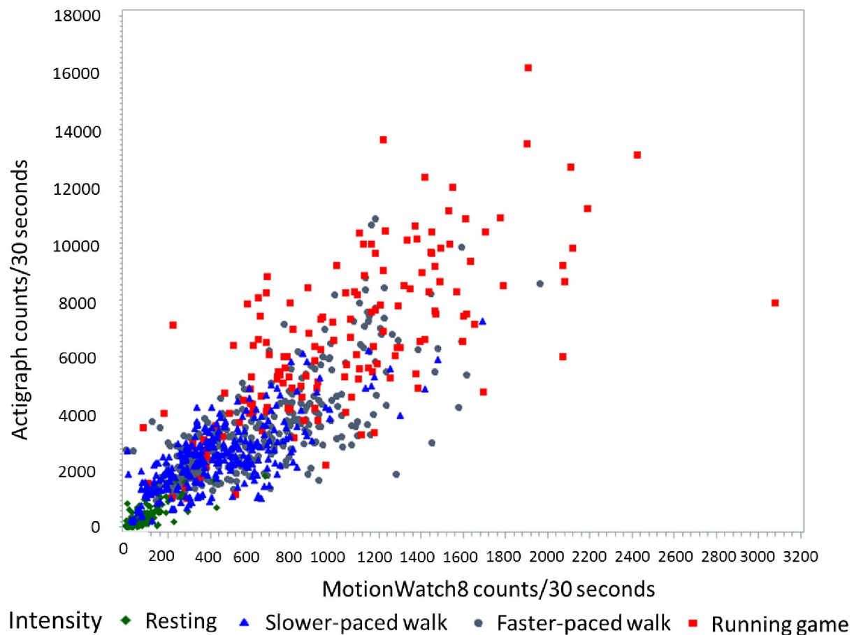
Fig 1. Correlation between mean output from the MotionWatch8 and ActiGraph accelerometers. The scatterplot demonstrates higher absolute counts of motion (acceleration) measured using the ActiGraph compared to the MotionWatch8, but positive correlation ( r = 0.85 , p < 0.001 ) between devices when worn in the same participants simultaneously. Each study participant contributed three or four points on the scatterplot to represent four different intensities of movement during a structured activity (Diamond: resting, triangle: slower-paced walk, dot: faster-walk, square: running game). Only 13 of the total 39 participants contributed data for the resting activity.
