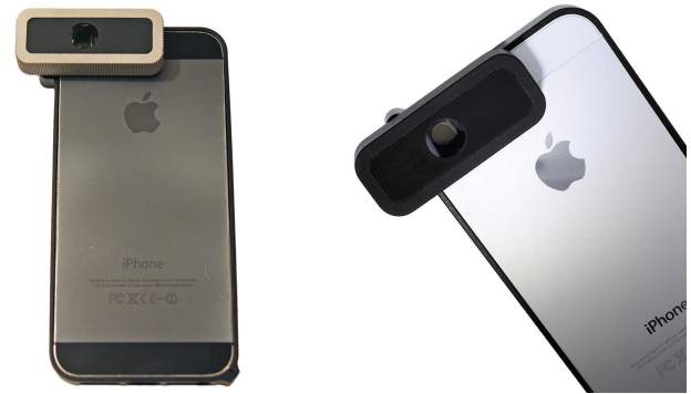
FIGURE 2: Picture of the prototypes magnetically attached to different iPhone (5 and 5s; Apple, Cupertino, CA) models.
