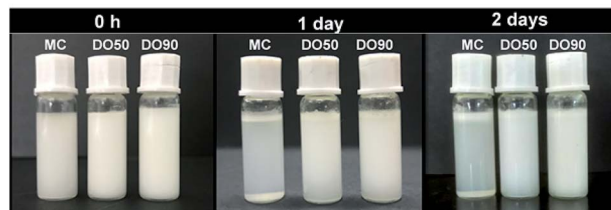
Fig. 6 Kinetic instability diagram (upper) and pictures (down) of MC, DO50 and DO90 stabilized Pickering emulsion in 24 h. Experiments were performed at least triplicate and no significant difference in the same sample ( P > 0.05 ). * p < 0.05 , ** p < 0.01 , *** p < 0.001 . The prepared Pickering emulsions (oil to water ratio is 1/10 (v/v)) in PBS of pH 7, ionic strength of 150 mM and the temperature was controlled at 25.0 \pm 0.5 °C.
