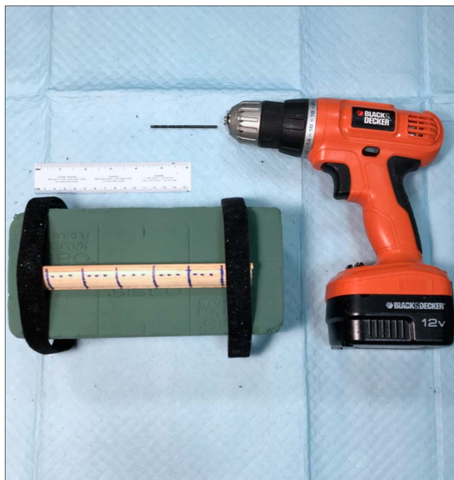
Fig. 2 Photograph of the depth of plunge simulation module.
