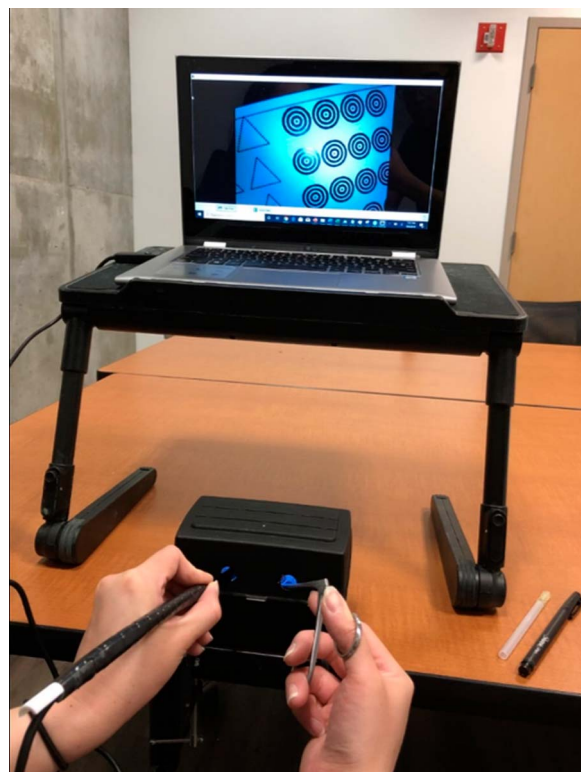
Fig. 8 Photograph of the wrist arthroscopy module with a laptop screen showing real-time feed of the simulated arthroscopic camera.
