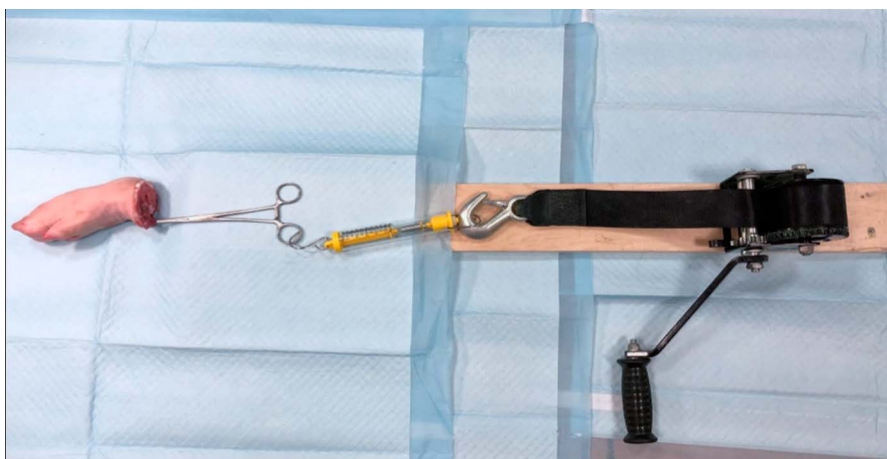
Fig. 3 Photograph of the flexor tendon repair simulation model and testing jig.
