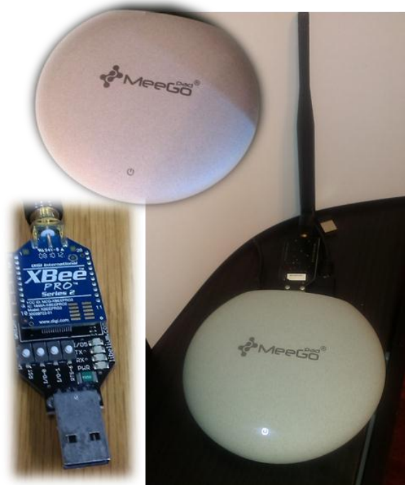
Figure 13. Infrastructure's hardware, including XBee Pro ZigBee Motes and MeeGo Mini PC sink device.
