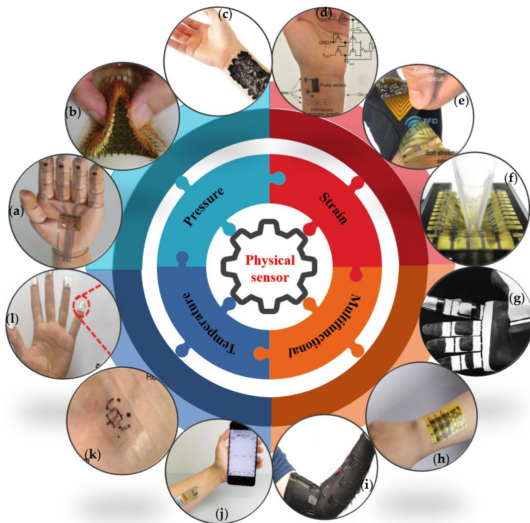
Figure 1. Representations of flexible physical sensors and typical applications: (a) A model hand with pressure sensor on the fingertips (Reprinted with permission from ref. [31]. Copyright 2015, American Association for the Advancement of Science); (b) Pressure–sensor integration attached to the surface of a soft balloon (Reprinted with permission from ref. [32]. Copyright 2019 Royal Society of Chemistry); (c) Leather-based e-skin with sensing capability by merging the sophisticated hierarchical structure of leather (Reprinted with permission from ref. [33]. 2018 The Authors); (d) Pulse signals measured by a stretchable strain sensor (Reprinted with permission from ref. [34]. Copyright 2018 Springer Nature); (e) Sensor for sensing the pulse on a human wrist (Reprinted with permission from ref. [35]. Copyright 2019, The Authors); (f) Skin-like stretchable strain sensor by poking with a plastic bar (Reprinted with permission from ref. [36]. Copyright 2019 The Authors); (g) Flexible multimodal sensor wrapped onto a finger of a robotic hand (Reprinted with permission from ref. [37]. Copyright 2016 American Association for the Advancement of Science); (h) The malleable e-skin can be comfortably mounted onto a human arm (Reprinted with permission from ref. [38]. Copyright The Authors); (i) Textile-based sensor-integrated sleeve for hand motion detection (Reprinted with permission from ref. [39]. Copyright 2020 The Authors); (j) Temperature sensor mounted on an arm for real-time body temperature monitoring (Reprinted with permission from ref. [40]. Copyright 2020 The Authors); (k) Stretchable integrated circuit for strain-independent temperature sensing (Reprinted with permission from ref. [41] Copyright 2018 The Authors); (l) Flexible temperature sensor attached to fingers of the hand for temperature sensing (Reprinted with permission from ref. [42]. Copyright 2019 WILEY-VCH Verlag GmbH & Co. KGaA, Weinheim, Germany).
