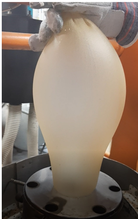
Figure 1. Starch-based film with functional substances blowing in laboratory.
