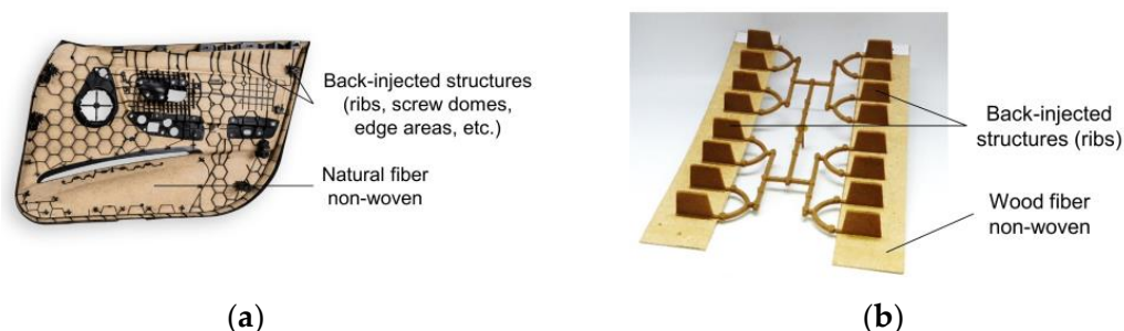
Figure 1. (a) State-of-the-art technology door panel from automotive interior made of a natural fiber non-woven with back-injected structures (ribs, screw domes, edge areas, etc.), image from Yanfeng Automotive Interiors with added labeling [16]; (b) test specimen for analyzing the bond strength via pull-off test, for a non-woven made of wood fibers (spruce) and PP, with the ribs back-injected onto the non-woven.
