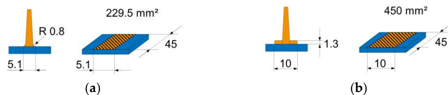
Figure 3. Two different rib geometries were molded for investigating the bond strength. (a) rib with radius; (b) rib with foot.
