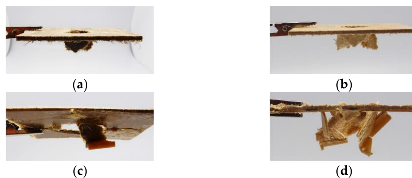
Figure 16. Exemplary specimen after impact test. (a) natural fiber non-woven; (b) wood fiber non-woven; (c) natural fiber non-woven with reinforcement rib (hybrid); (d) wood fiber non-woven with reinforcement rib (hybrid).
