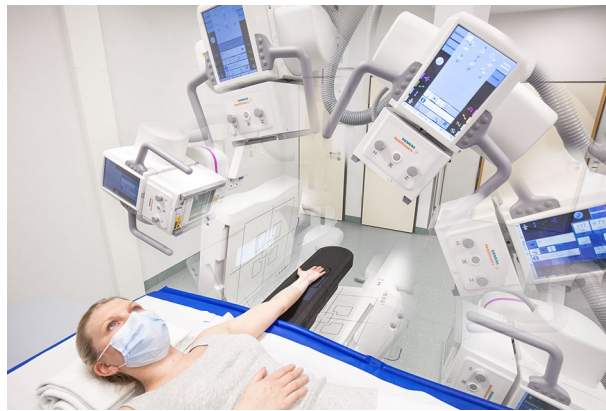
Figure 1. Rendering of staff member demonstrating the scan position for 3D cone-beam CT imaging of upper extremity joints using the tableside trajectory of the twin robotic x-ray system.
