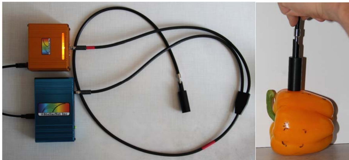
Figure 3. Light reflectance measurements (0° from the normal) with a portable spectrometer.
