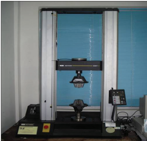
Figure 5: Universal testing machine - Instron 5567 compression tension tensile meter used to dislodge the overdentures from the models
