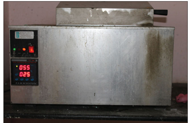
Figure 7: Manual thermocycling unit S-U-Polytub, Schuler Dental, Germany
