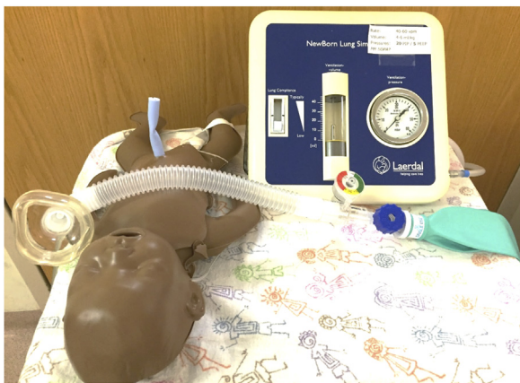
Fig. 2 – PPV-Refreshers: Image of infant training manikin with Newborn Lung Simulator (NLS), flow-inflating bag and infant mask on a mobile cart. The console provides visual feedback on PPV volume (mL, center cylinder) and pressure (mmHg, right analogue dial). Providers practiced until PPV competence (defined as PPV volume 10–21 mL and rate 40–60 vpm) could be demonstrated for at least 30 s. Providers were coached and remediated, as needed, during their PPV-Refresher.
