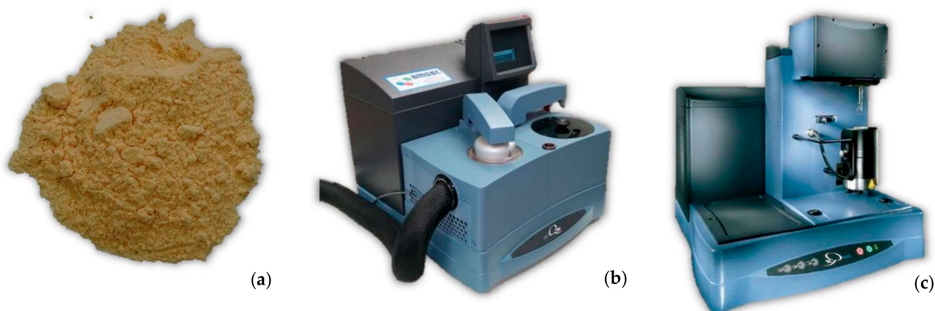
Figure 7. A-IX-1 explosive composition extracted from the PG-7VM warhead (a) to test on a differential scanning calorimeter DSC Q100 (b) and thermogravimetric analyzer TG Q50 (c).
