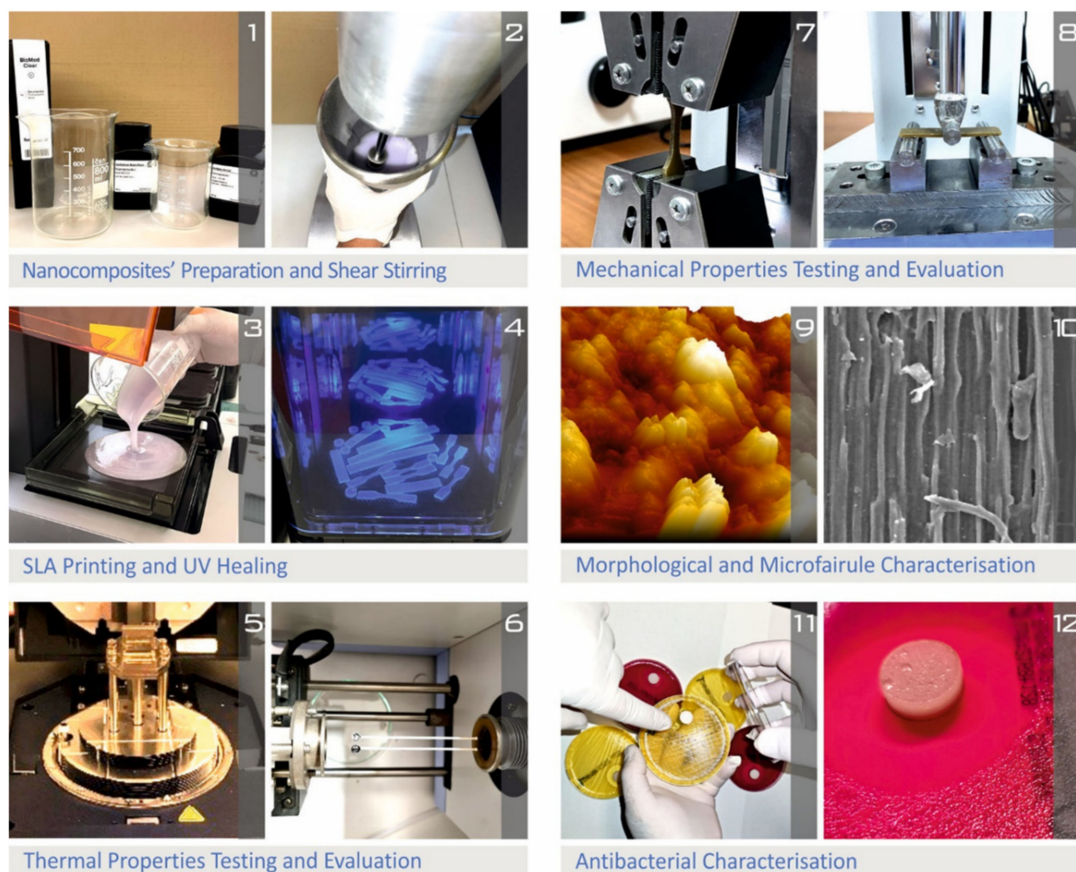
Figure 1. Flow chart illustrating the methodology followed to fabricate the different nanocomposites, as well as representative characterization techniques: (1) The additives used in this work, (2) materials mixing, (3) materials feeding in the 3D printer, (4) 3D printing process, (5) Mechanical testing (DMA), (6) Thermal properties (TGA), (7) Mechanical testing (tensile test), (8) Mechanical testing (flexural test), (9) morphological analysis (AFM), (10) morphological analysis (SEM), (11) (well agar diffusion), (12) antibacterial tests (inhibition zone).
