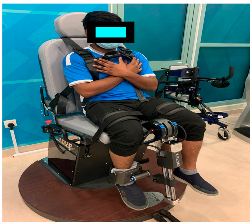
Figure 2. Measurement of the maximal voluntary isometric contraction at 90° using an ISO-MOVE isokinetic dynamometer.
