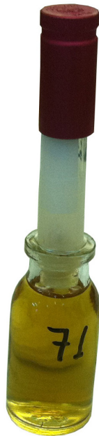
Fig. 1. Two-chamber device for bacterial leakage.
