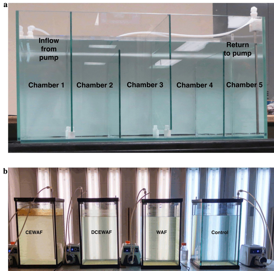
Fig. 1. (a) Baffled Recirculating Tank. Each chamber is numbered chambers 1–5 from the left; (b) 110L Mescosm tanks used for Marine Oil Snow experiments.
