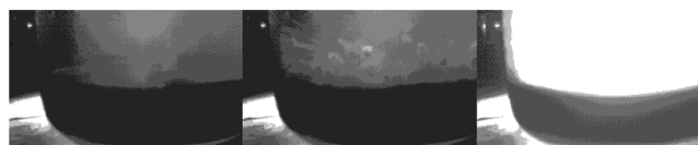
Figure 3. Ignition process of fuel and NTO: fuel contact with NTO liquid surface; white fog production; and ignition.
