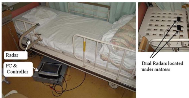
Fig. 21. The radar equipment of a non-contact bedside autonomic activation monitoring system. Dual 24-GHz microwave radars are attached beneath the mattress of the patient's bed. [117].
