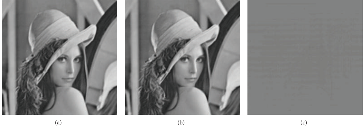
FIGURE 2: An example of reconstruction of image from local phase information. (a) Original image, the dimension of the space is 16,129. (b) Reconstructed image from 20,102 phase measurements, scaled to match the original. (c) Error.
