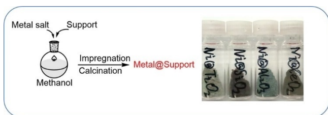
Figure 1. General preparation of supported 3d-metal-based catalysts.
