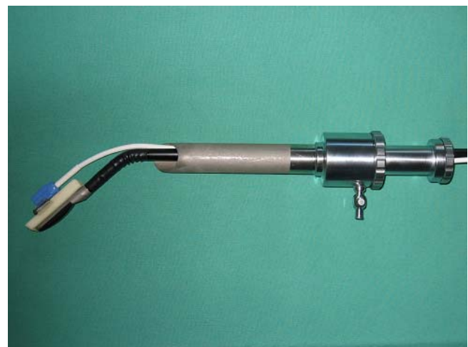
Figure 2 LUS connected to the navigation system US Guide 2000® inserted through a 22 mm trocar in an experimental environment.
