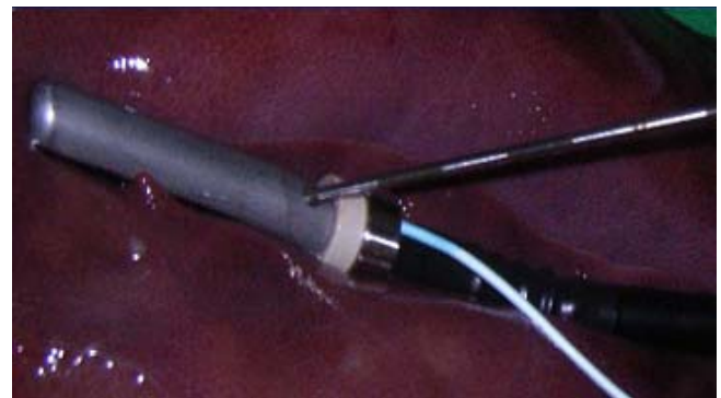
Figure 5 Connection of LUS transducers with AURORA® electromagnetic tracking by the "ring" adapter.
