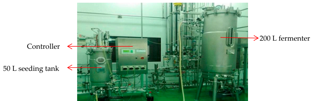
Figure 14. Illustration of the E. coli fermentation system.
