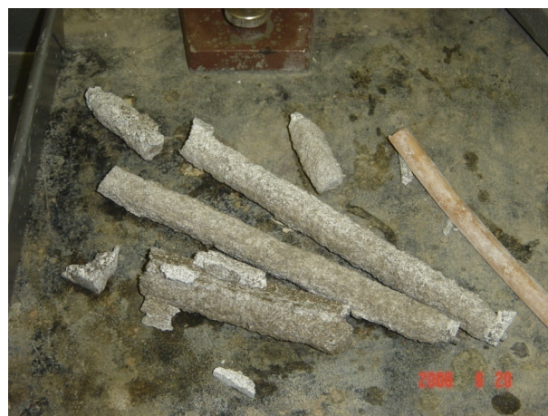
Figure 2. Mortar bars severely deteriorated after immersion in NaOH solution for 63 days.
