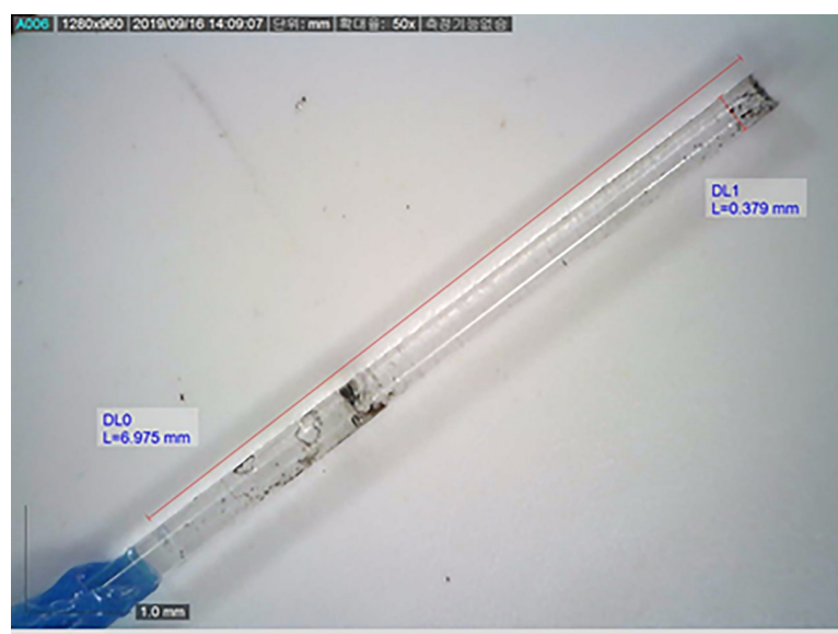
Fig 4. Fiber was stripped to measure the length of fiber core degradation.
