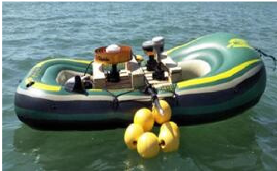
Figure 11. Dynamic test carried out by using Trimble R10 receiver on an inflatable boat.
