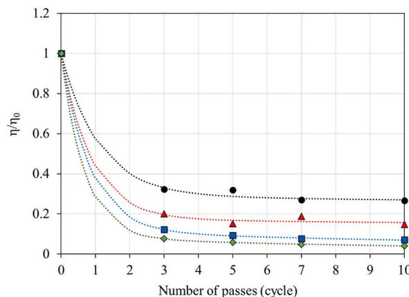
Fig. 5. Plot of the normalized apparent viscosity ( $\eta/\eta_0$ ) as a function of number of passes through the microfluidizer at 20,000 psi in the case of  $\beta$ -glucan suspensions of 0.5% w/w (●), 1% w/w (▲), 2% w/w (■), and 3% w/w (◆) solid concentrations.
