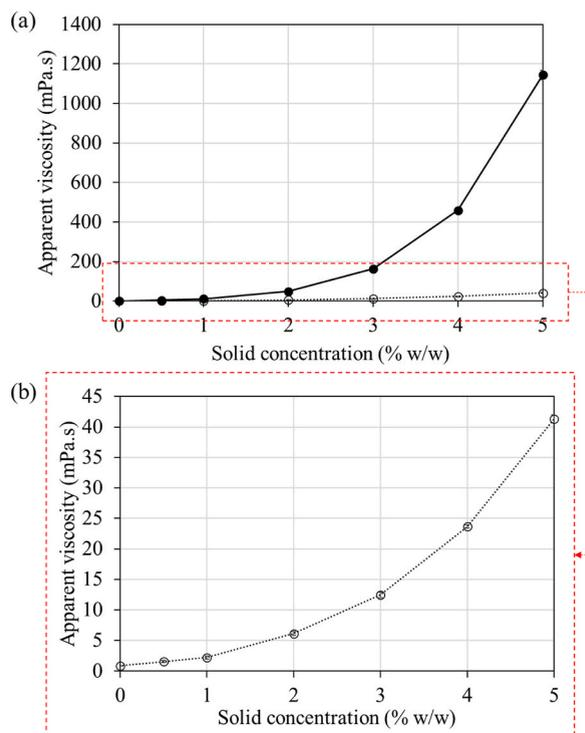
**Fig. 4.** Dependence of the apparent viscosity of a suspension of  $\beta$ -glucans secreted by *Ophiocordyceps dipterigena* BCC 2073 on the  $\beta$ -glucan solid concentration determined before (solid line) and after (dotted line) the suspension underwent fragmentation conducted at 20,000 psi over three cycles.
