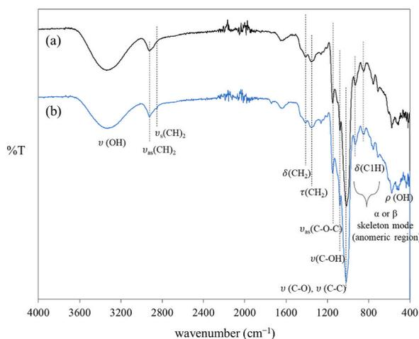
**Fig. 6.** Fourier-transform infrared spectra of suspensions of  $\beta$ -glucans secreted by *Ophiocordyceps dipterigena* BCC 2073 recorded (a) before and (b) after fragmentation.
