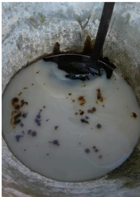
Fig. 5. Photograph of the DNAPL in emulsion extracted at the sampling point located at the bottom of the alluvium (16 m b g.l.) in well PS14D 40 min after the injection had stopped.
