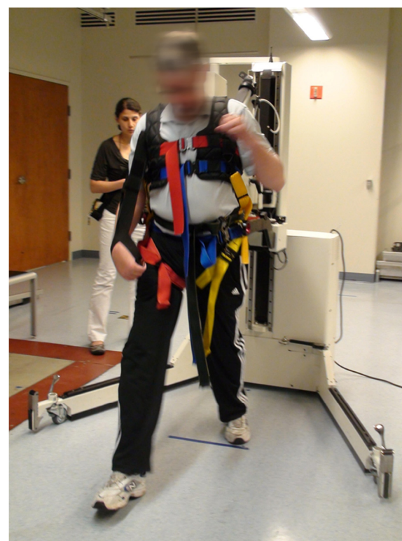
Figure 1 Overground robotic gait and balance system (KineAssist TM ) use to provide external forces at the pelvis during walking (i.e. "push mode" walking).
