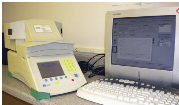
Figure 1. Bio-Rad iCycler thermocycler unit (Bio-Rad, Hercules, CA USA) with real-time computer interface (Courtesy Veterinary Molecular Diagnostics, Inc.).
